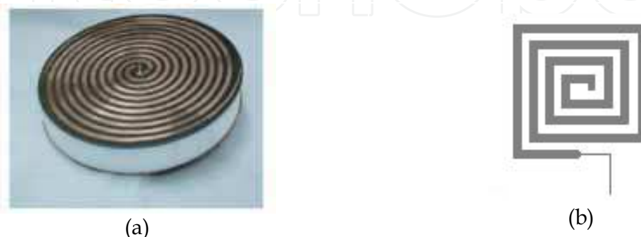
Fig. 8. a) Structural pattern of the microstrip circular spiral printed antenna b) Sketch of the rectangular spiral antenna
