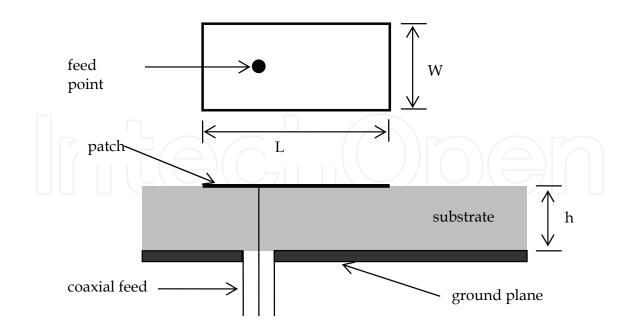
Fig. 1. Geometry of rectangular MSA
