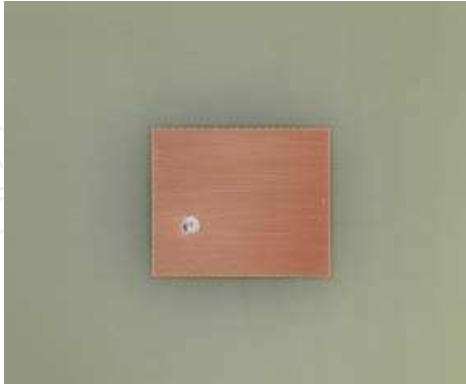
Fig. 21. Photo of the CP microstrip antenna prototype.
