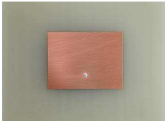
Fig. 19. Photo of the LP microstrip antenna prototype.
