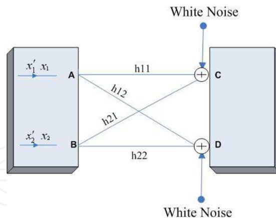
Fig. 1. General architecture of a MIMO 2×2.
