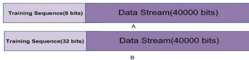
Fig. 16. The burst of LS-based SBCE-ML. A) MIMO 2x2, B) MIMO 4x4.
