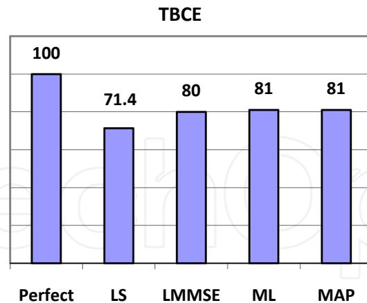
Fig. 5. Relative processing time of different estimators with respect to perfect one in a MIMO 2x2 (TBCE).
