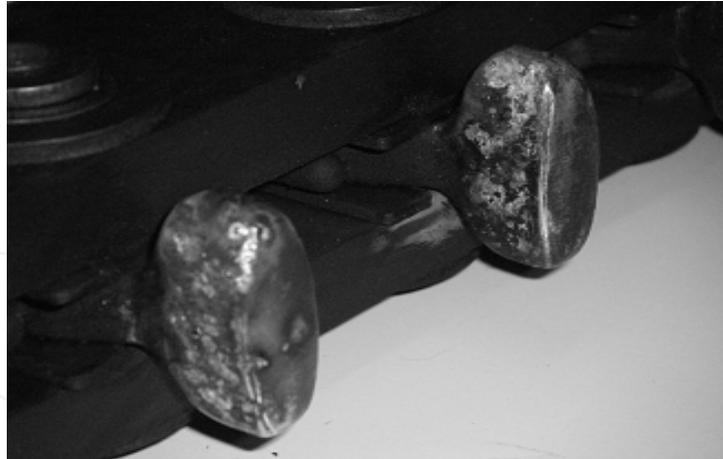
Fig. 5. Tap selector fixed contacts damaged by arcing
