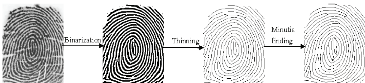
Fig. 3. Output images of PS1802 modalafs minutia extraction algorithm.
