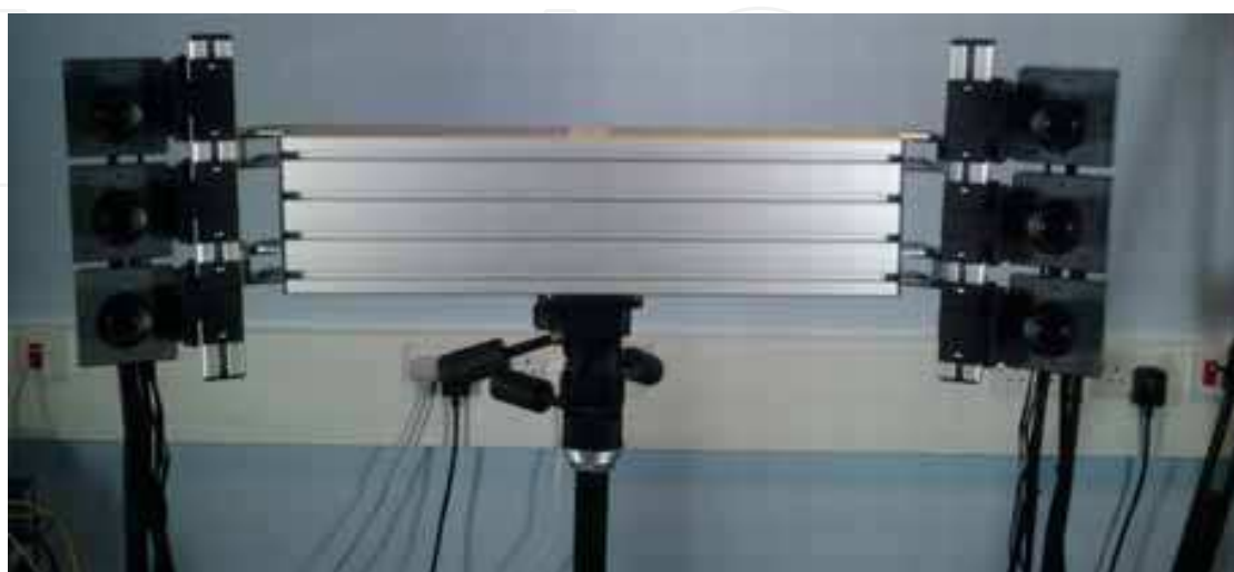
Fig. 3. A passive 3-D scanner from Dimensional Imaging.
