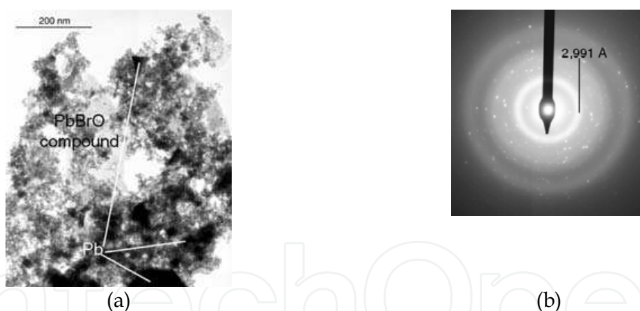
Fig. 10. (a) TEM observation of washed lead salt reduction powder, (b) corresponding electron microdiffraction pattern of the Pb x Br y O z compound
