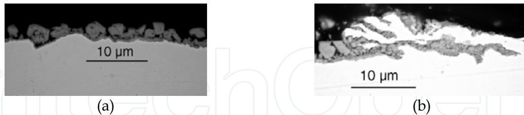
Fig. 27. Cross sections after cyclic corrosion test ( 1\text{A.dm}^{-2} ) of the lead coating annealed at 80^\circ\text{C} (a), at 110^\circ\text{C} (b) (local infiltrations of corrosion products under the coating)
