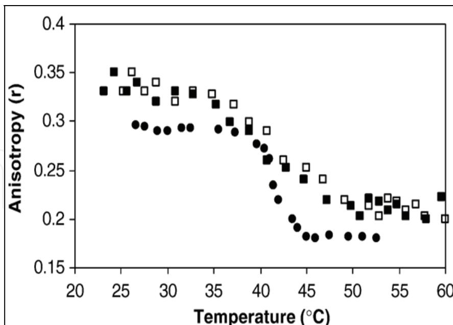
Fig. 7. Liposomes transition temperature from DPH fluorescence polarization: a) DPPC liposomes ( $\bullet$ ); b) as-synthesized DPPC liposils ( $\blacksquare$ ); c) DPPC liposils after the kinetics in acidic fluid ( $\square$ )
