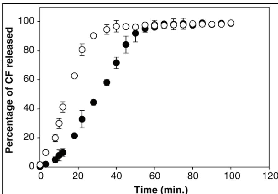
Fig. 8. Kinetics profiles for the release of 5,6-CF from the composite silica nanoparticles in suspension at pH 7.4 for 90 min: a) DPPC liposils ( $-\circ-$ ); b) DPPC:chol liposils ( $-\bullet-$ )
