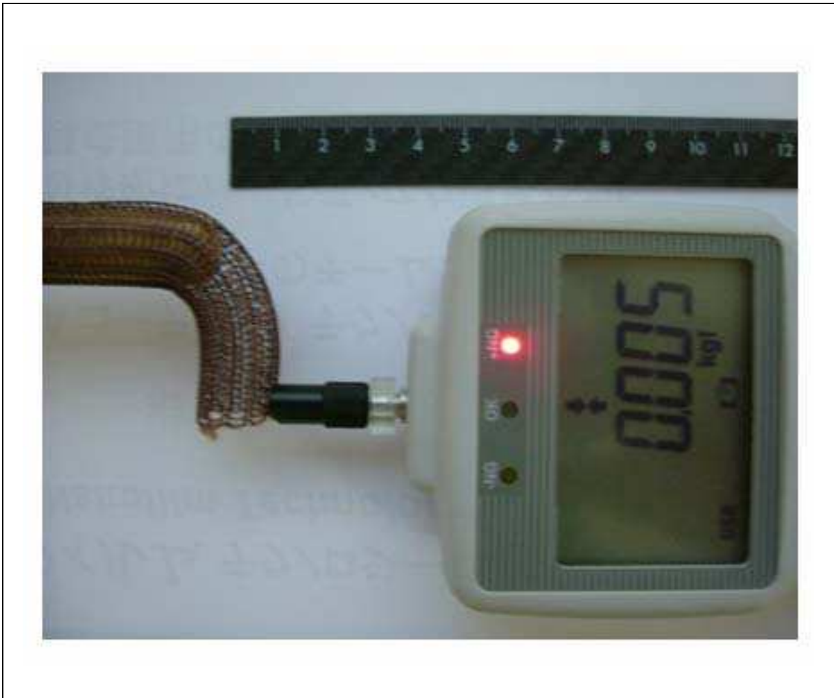
Fig. 9. With a mandrel inserted at one end of each stent, the other end was contacted by a push-pull gauge (IMADA Co., Aichi, Japan) on the surface of the stent, and was given external force until the stents were bent to an angle of 90 degrees. The value of the weight on the gauge was defined and measured as the bending force of the stent
