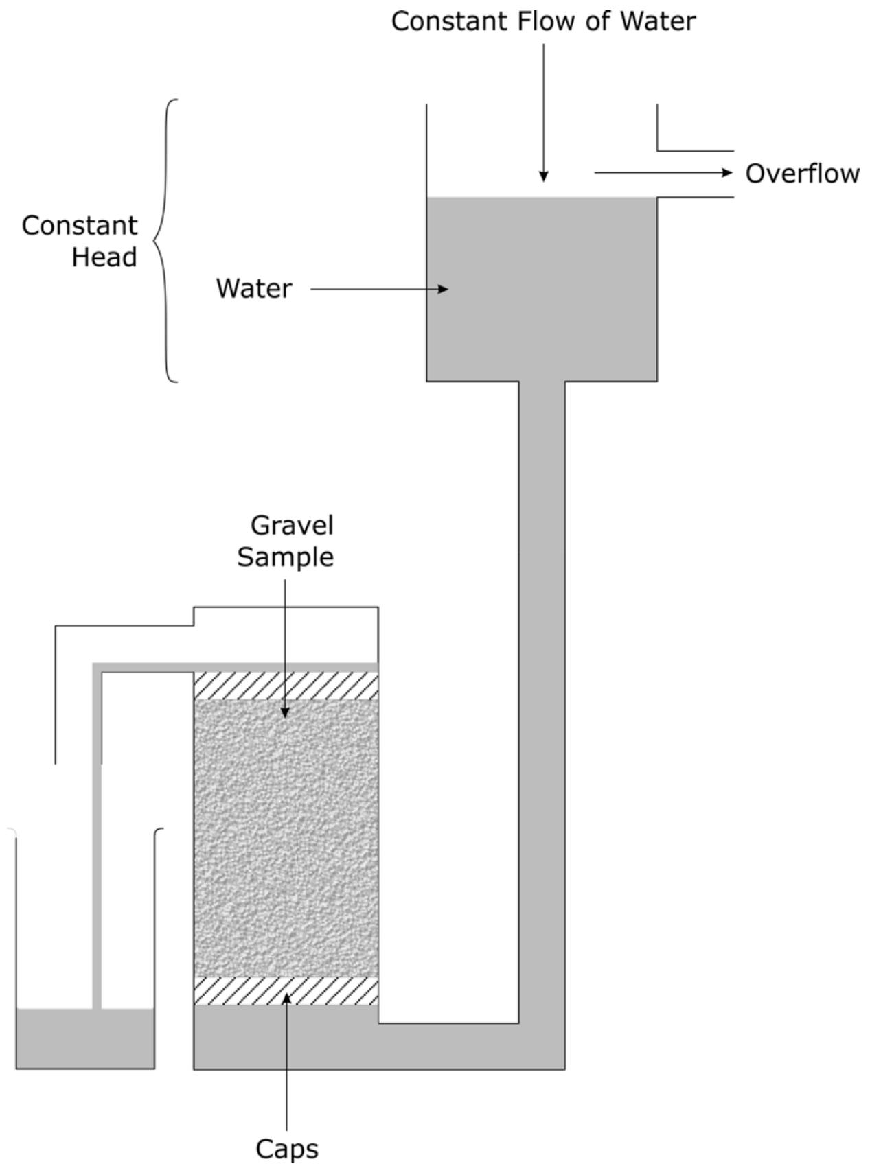
Fig. 5. Schematic representation of laboratory permeameter setup.
