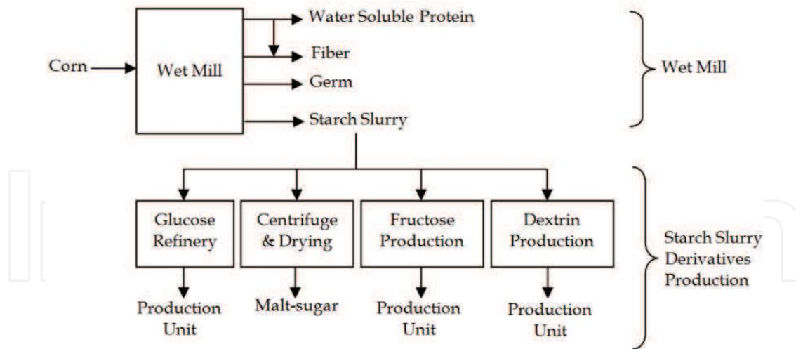
Fig. 3. Process flow diagram for a typical corn processing industry
