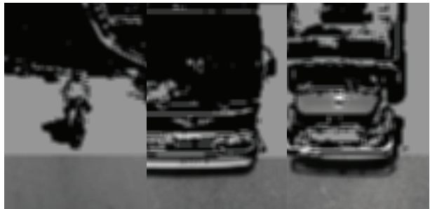
Fig. 6. Vehicle images after applying histogram equalization
