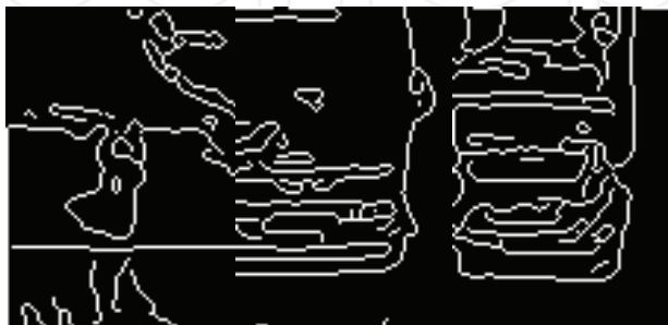
Fig. 7. Vehicle images after applying Canny edge detection
