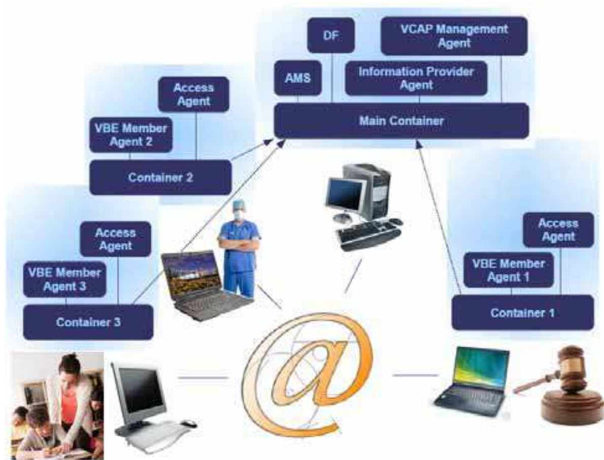
Fig. 9. Distributed structure of the VCAP platform
