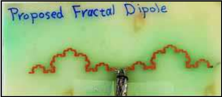
Fig. 10. Photograph of the fabricated (P3) antenna
