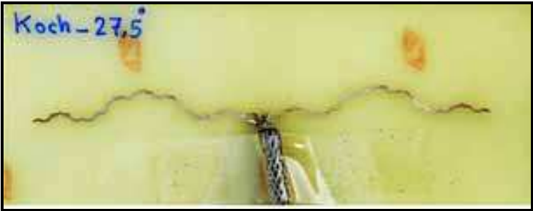
Fig. 9. Photograph of the fabricated K3-27.5° antenna.
