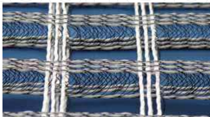
Fig. 23. Net spacer used for textile reinforced concrete
