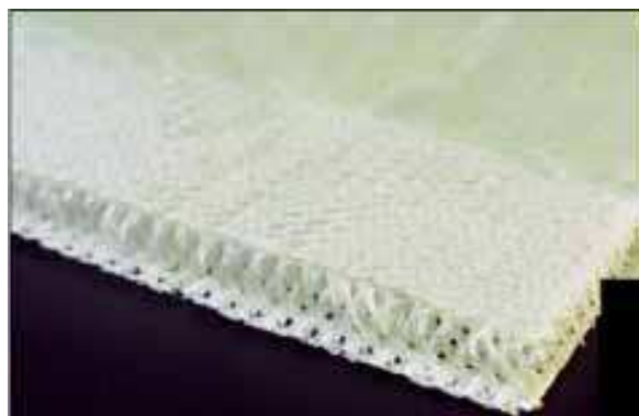
Fig. 22. Spacer fabric made of glass fibre
