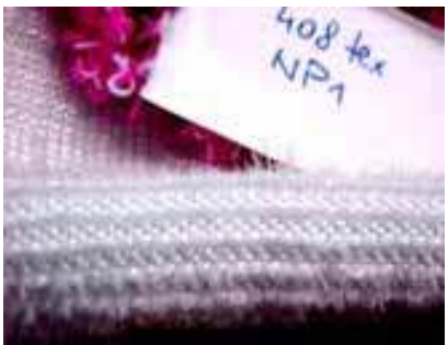
Fig. 5. Aspect of the jersey fabric (408 tex) knitted with NP1=10.5
