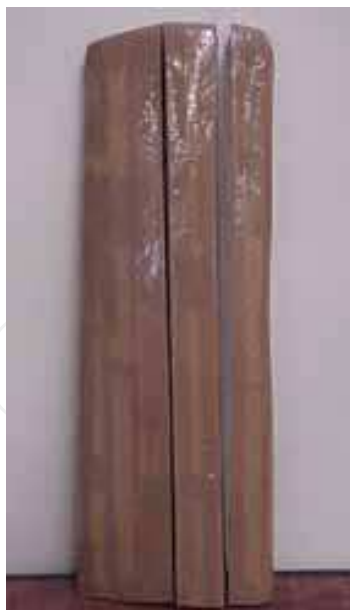
Fig. 42. Exterior mould – inferior and superior components
