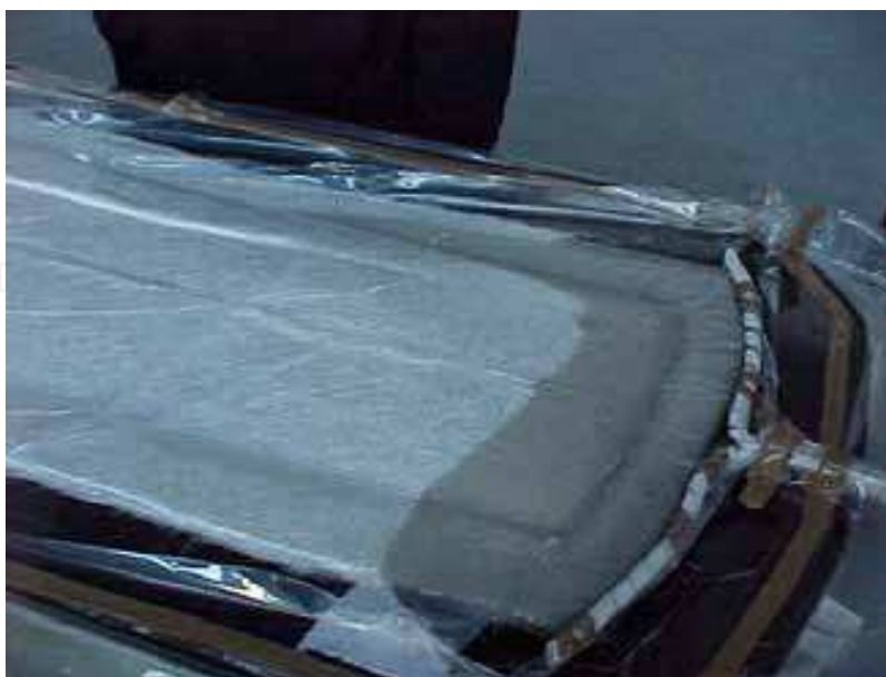
Fig. 45. Resin injection process
