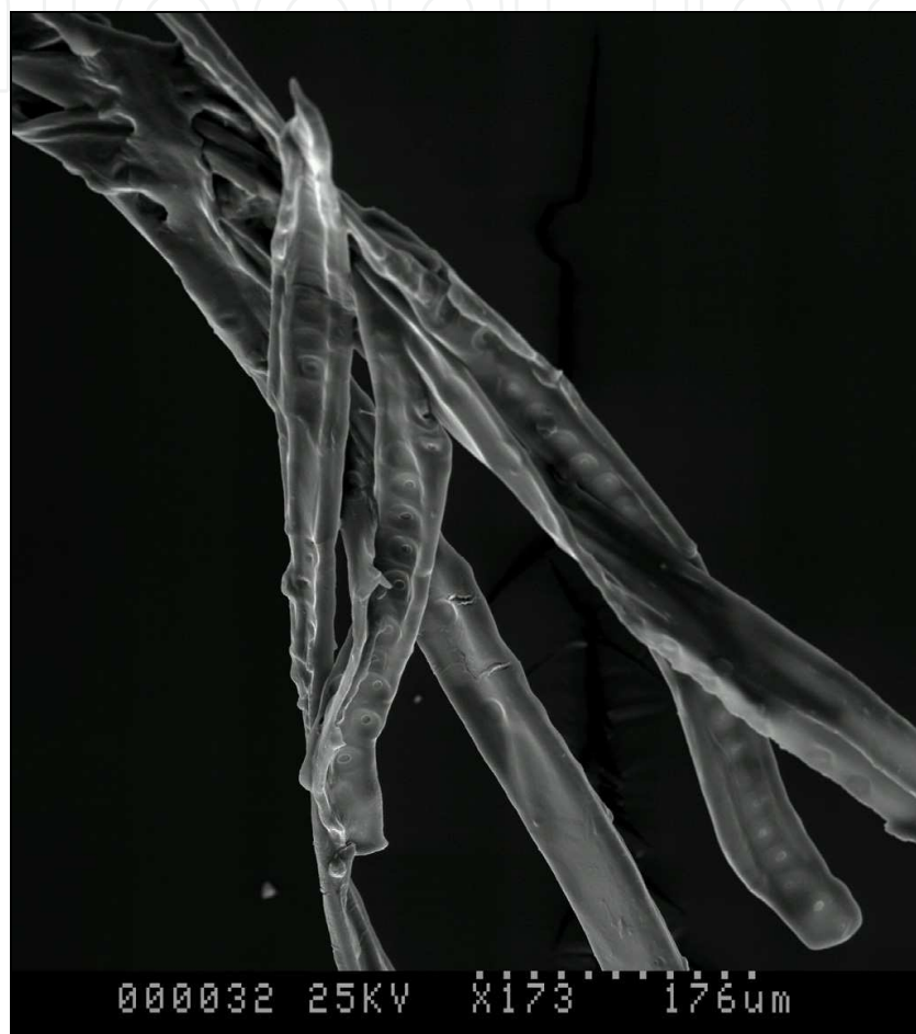
Fig. 7. Treated pine sapwood whose tracheids are easily manually disjoined
