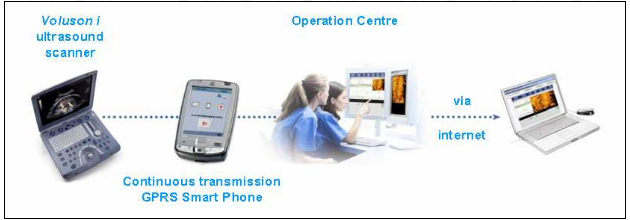
Fig. 2. Organization of the new TOCOMAT network for Tele-Ultrasonography.
