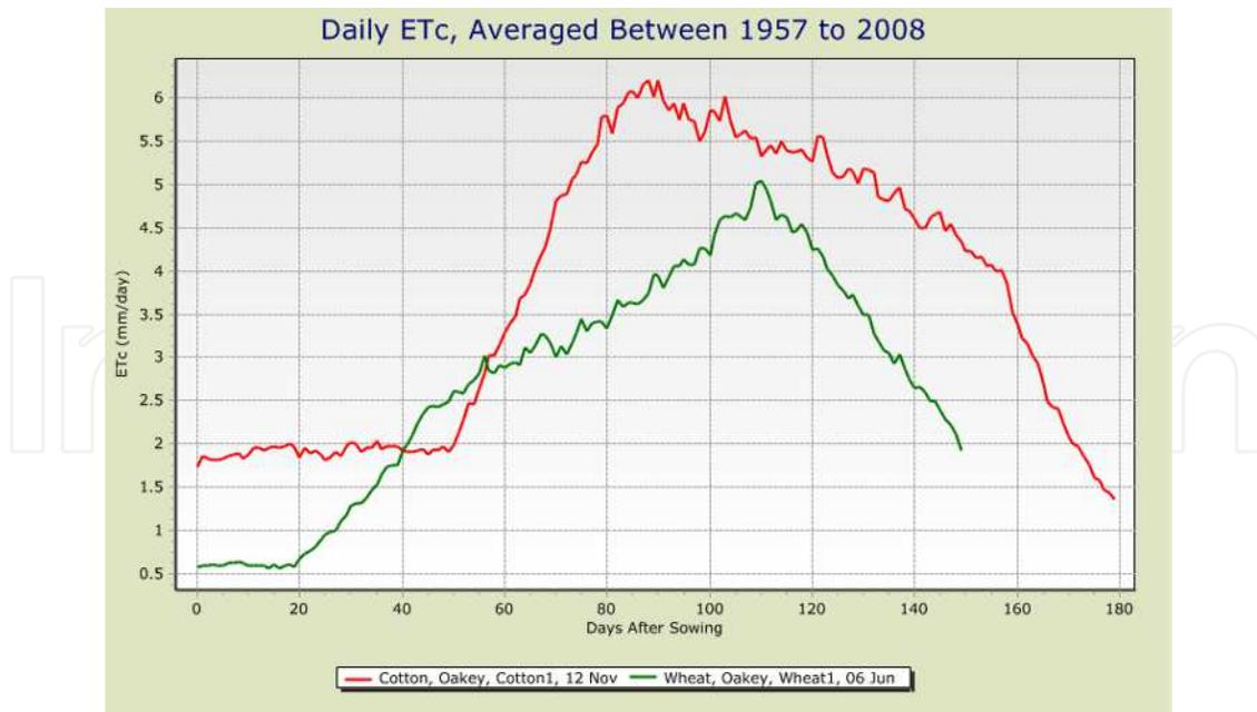
Fig. 4. Calculated average daily crop evapotranspiration as a function of days after sowing for cotton and wheat at Oakey
