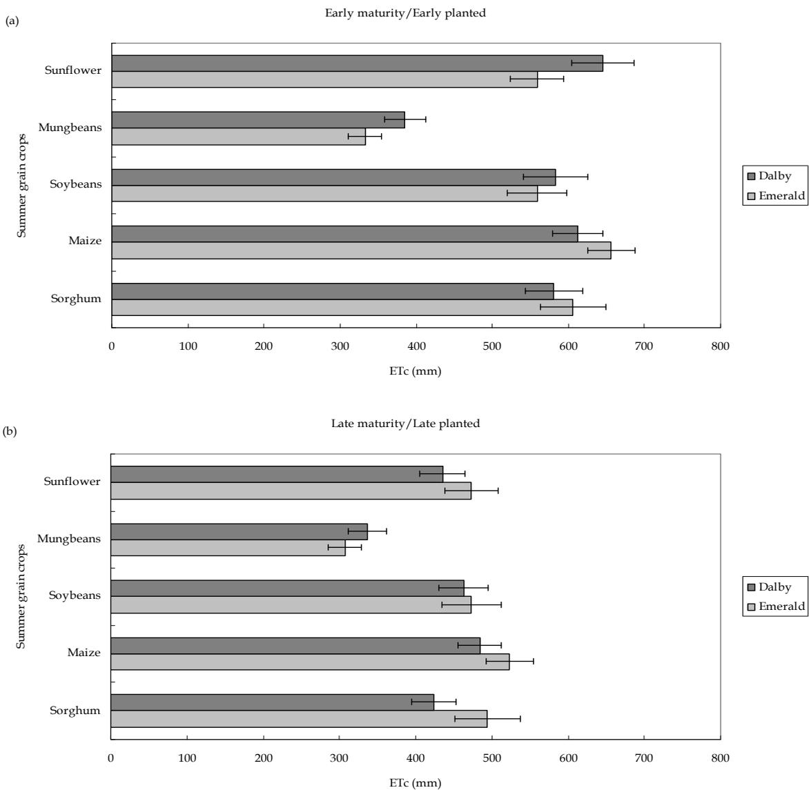
Fig. 14. Range of crop evapotranspiration (ETc) as estimated by the *CropWaterUse* tool using historical weather data (1957-2008) for “fully irrigated” sunflower, mungbeans, soybeans, maize and sorghum for various scenarios (a) early planting, early maturing varieties, and (b) late planting, late maturing varieties in cooler (at Dalby) and hotter (at Emerald) climatic conditions in Queensland. Bar indicates +/- standard deviation
