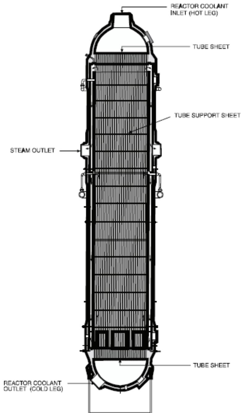
Fig. 3c. Typical Babcock & Wilcox Once through steam generator
