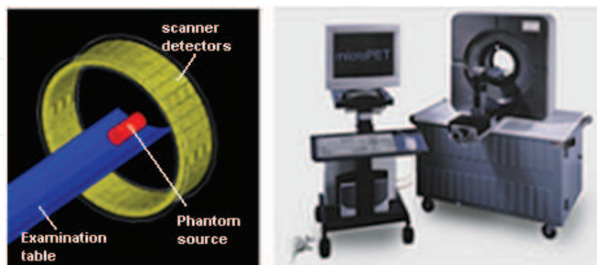
Fig. 1. MicroPET® FOCUS 220 geometry modeled by GATE (left) and the real system (right).
