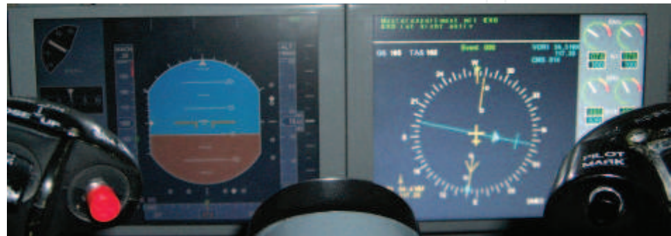
Fig. 2. Typical primary flight display and navigation display
