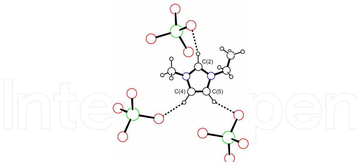
Fig. 2. Interionic contacts between  $C_2MI$  cation and  $Fe^{III}Cl_4$  dianion in  $[C_2MI]_2[FeCl_4]$ . Short C-H...Cl contacts are shown by dashed lines. The crystal structure was determined by a synchrotron X-ray powder diffraction measurement (Yoshida et al., 2005b).
