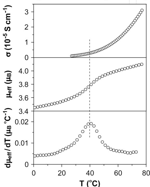
Fig. 6. Temperature dependence of ionic conductivity ( $\sigma$ ), effective magnetic moment ( $\mu_{\text{eff}}$ ), and its derivative  $d\mu_{\text{eff}}/dT$  of  $[P_{14,6,6,6}]_2[Co(DBSQ)_2(bpy(COO)_2)]$ . A vertical dotted line indicates the equilibrium temperature (Yoshida et al., 2009).
