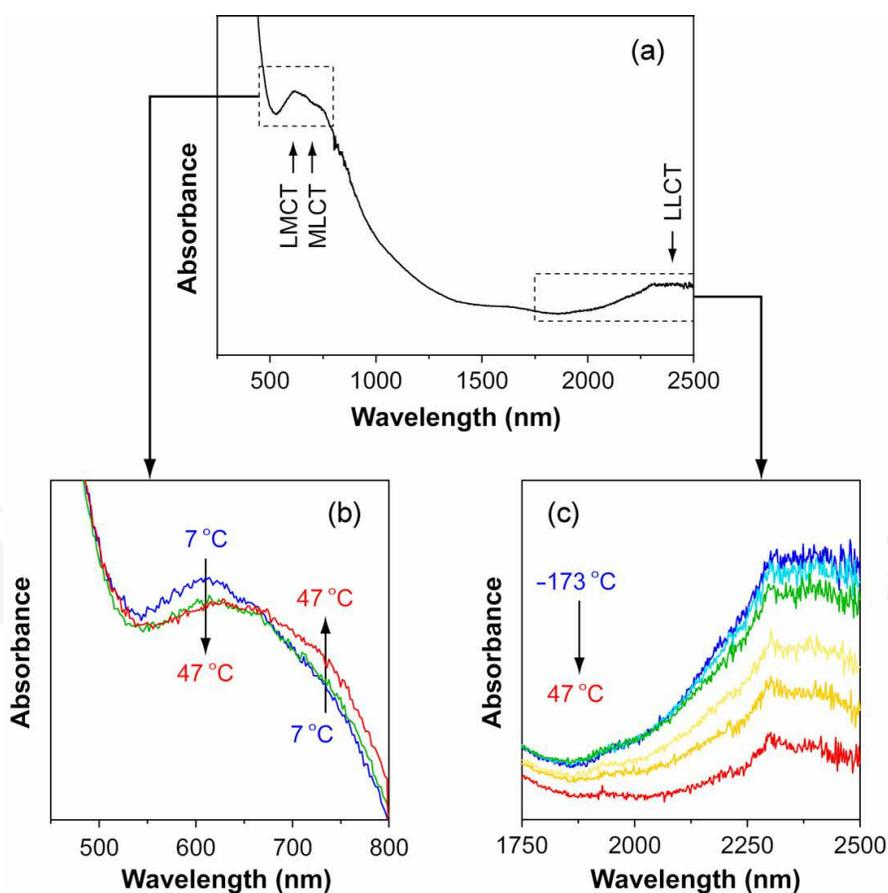
Fig. 5. (a) Electronic absorption spectrum of  $[\text{P}_{14,6,6,6}]_2[\text{Co}(\text{DBSQ})_2(\text{bpy}(\text{COO})_2)]$  at  $-173$  °C. Temperature dependence of the spectra (b) in the high-energy region (7, 27, 47 °C) and (c) in the low-energy region ( $-173, -73, -13, 7, 27, 47$  °C) (Yoshida et al., 2009).
