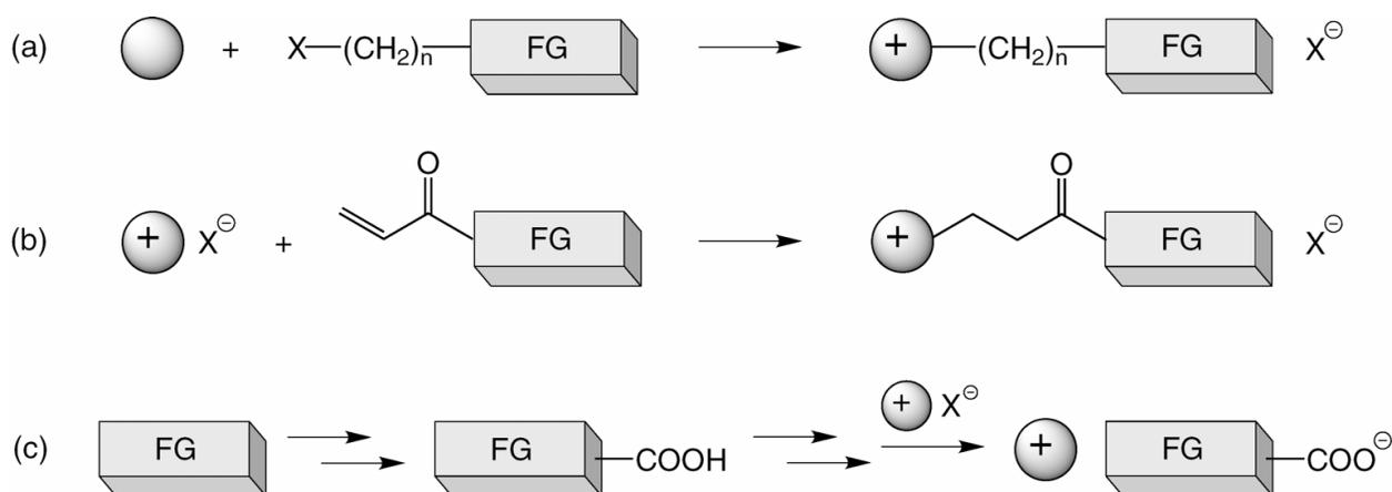
Scheme 2. Schematic synthetic routes of functional ionic liquids by (a) *N*-alkylation reaction (Davis, 2004) and (b) Michael addition reaction (Wasserscheid et al., 2003) to form ionic liquids of functional cations, and (c) the addition of acidic group to form ionic liquids of functional anion. A blank sphere represents a Lewis base such as imidazole, amine, phosphine, and sulfide, while a sphere with a plus sign represents the corresponding cation.
