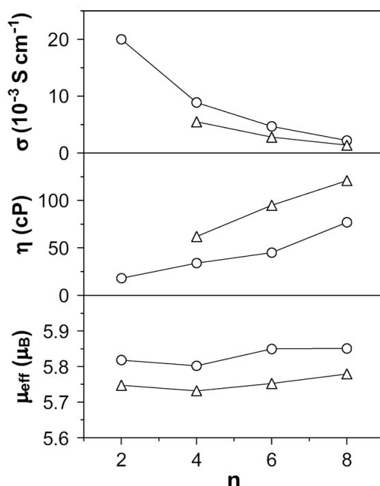
Fig. 3. Dependence of ionic conductivity ( $\sigma$ ), viscosity ( $\eta$ ), and effective magnetic moment ( $\mu_{\text{eff}}$ ) on alkyl chain length in the  $C_n\text{MI}$  cations for  $[C_n\text{MI}][\text{FeCl}_4]$  ( $\circ$ ) and  $[C_n\text{MI}][\text{FeBr}_4]$  ( $\Delta$ ) salts (Yoshida et al., 2005b; Yoshida & Saito, 2006).
