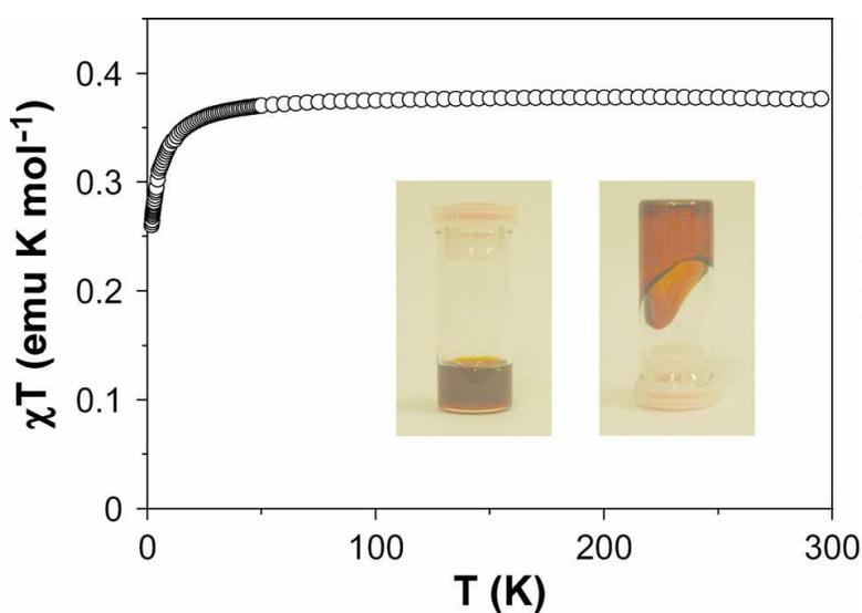
Fig. 4. Temperature dependence of the product of static susceptibility and temperature ( $\chi T$ ) for  $[C_4MI][TEMPO-OSO_3]$  in an applied field of 1 kOe on heating process. The inset is the photographs of  $[C_4MI][TEMPO-OSO_3]$  (Yoshida et al., 2007c).
