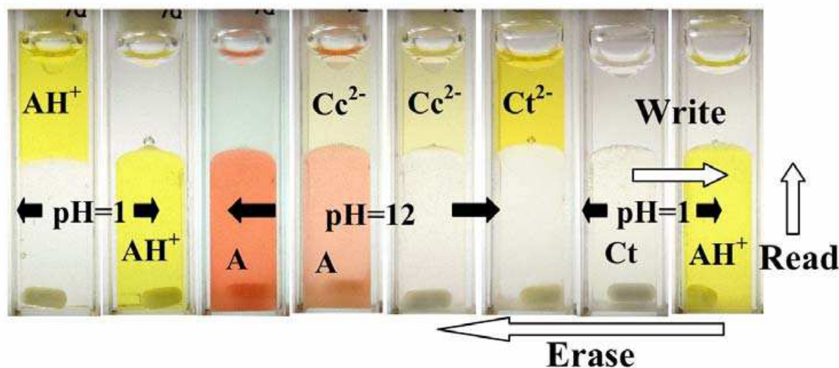
Fig. 4.3 - See from left side: a - [BMIM][PF 6 ] (bottom phase) and 4'-hydroxyflavylium perchlorate in 0.01 M HCl (upper phase); b - after strong shaking of both solutions; c - after alkalinisation of the aqueous phase (pH≈12) with minimum shaking; d - after medium shaking; e - after strong shaking; f - after several minutes at room temperature or upon irradiation of the aqueous phase; g - after reacidification of the aqueous phase (pH≈1) and strong shaking; h - after irradiation of the ionic liquid phase.
