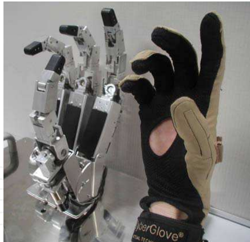
Fig. 10. A data glove controlling the joints motion of a robotic hand
