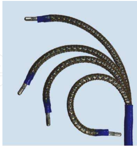
Fig. 4. A continuum manipulator with tendon actuation
