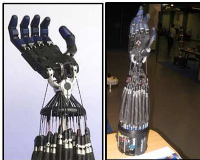
Fig. 6. The Shadow hand actuated with air muscles
