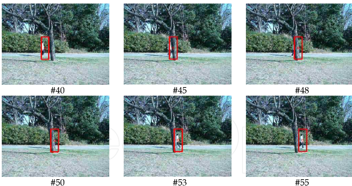
Fig. 17. Object tracking in the presence of occlusion
