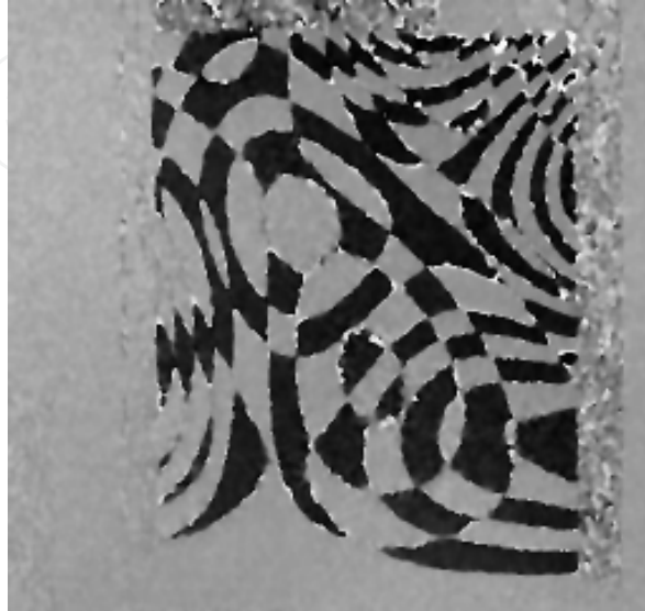
Fig. 12. Phase difference with compensated \Delta\varphi_{o-r}
