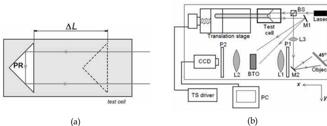
Fig. 14. (a) - 90°-prism retro reflector PR in test cell; (b) - Optical setup for the holographic refractometer : BTO,  $\text{Bi}_{12}\text{TiO}_{20}$  crystal; BS, beam splitter; M1 and M2, mirrors; P1 and P2, polarizers; L1 to L3, lenses; translation stage TS driver , CCD camera and PC computer for image acquisition (Barbosa et al, 2010).
