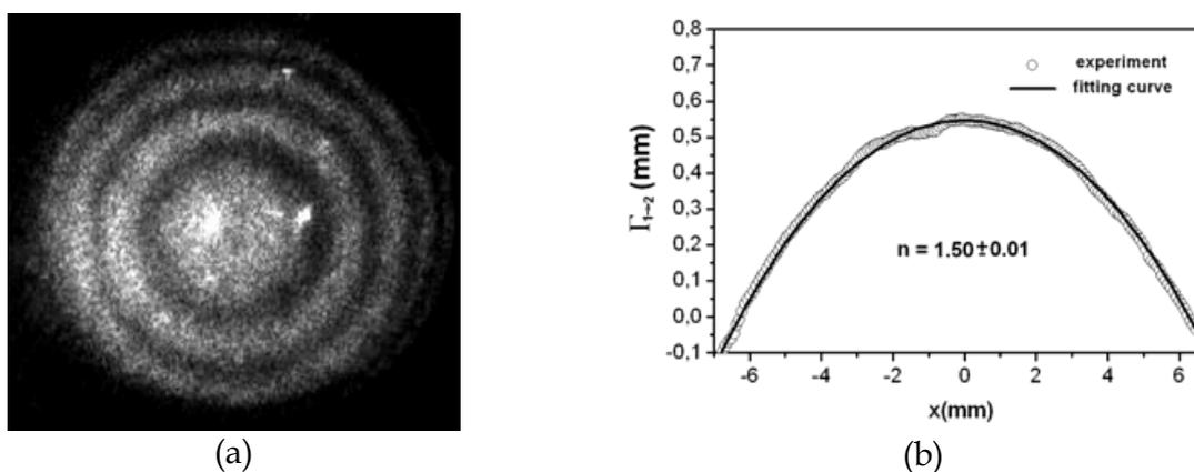
Fig. 17. (a) - Contour fringe pattern for  $\Delta z = 0.24$  mm when the illuminating beam traveled through the lens; (b) - averaged  $y$ -coordinate of the reconstructed wavefront providing  $n = 1.50 \pm 0.01$  (Barbosa et al, 2009).
