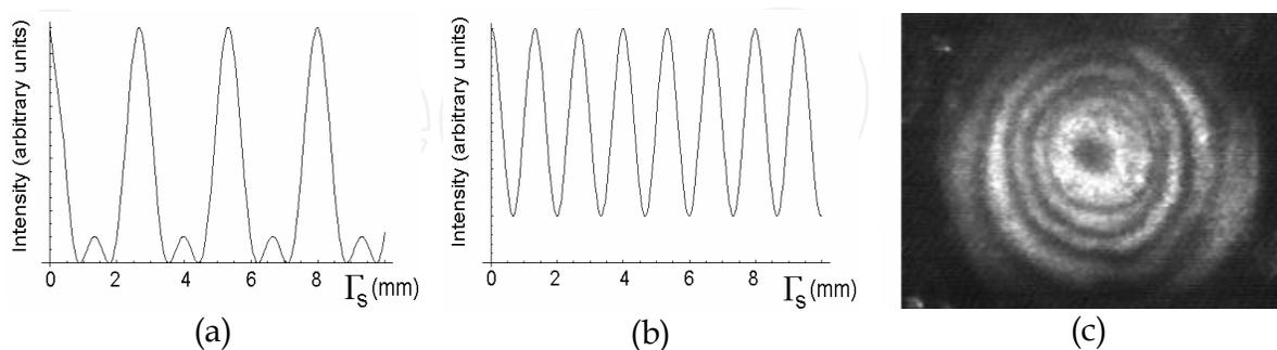
Fig. 6. - Interferogram intensity distribution as a function of  $\Gamma_S$  for holographic recording with (a) - one reference beam and (b) - two reference beams; (c) - Holographic image of the loudspeaker generated by a two-reference beam setup (Barbosa et al, 2005)
