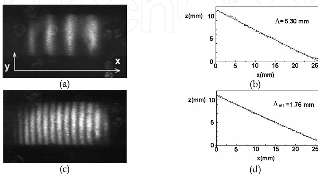
Fig. 7. Profilometry of a tilted plate. (a) - Interferogram for  $\lambda_S = 5.30$  mm and  $\Delta z = 2.65$  mm; (b) - corresponding profile; (c) - Interferogram for  $\lambda_S = 1.76$  mm and  $\Delta z = 0.88$  mm; (d) - profile of the same section (Barbosa et al, 2007).
