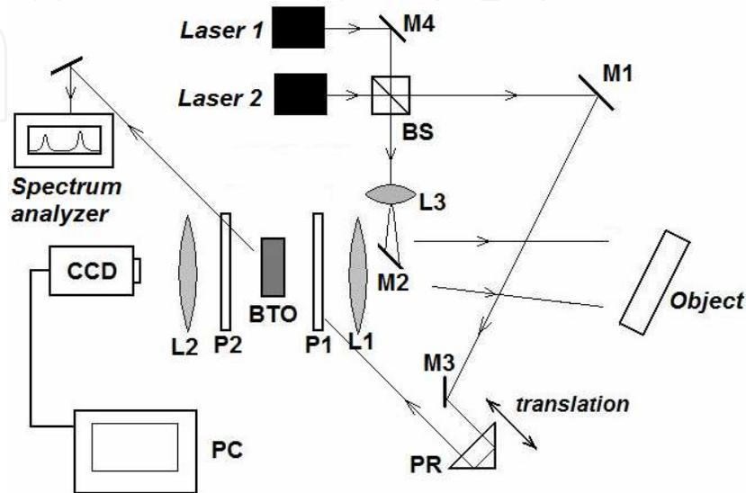
Fig. 8. Two-laser holographic interferometer
