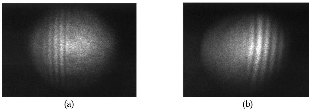
Fig. 12. Two-wavelength holographic imaging of the V-shaped surface by focusing the fringe pattern of (a) - the left half ( $x' > 0$  and  $\partial H/\partial x' < 0$ ) of the surface, and (b) - the right half of the surface ( $x' < 0$  and  $\partial H/\partial x' > 0$ ) (Barbosa, 2010)
