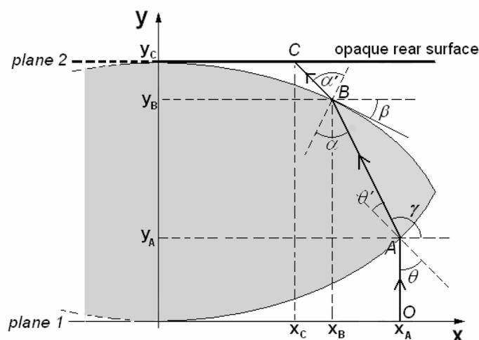
Fig. 15. Beam propagation through the spherical test lens
