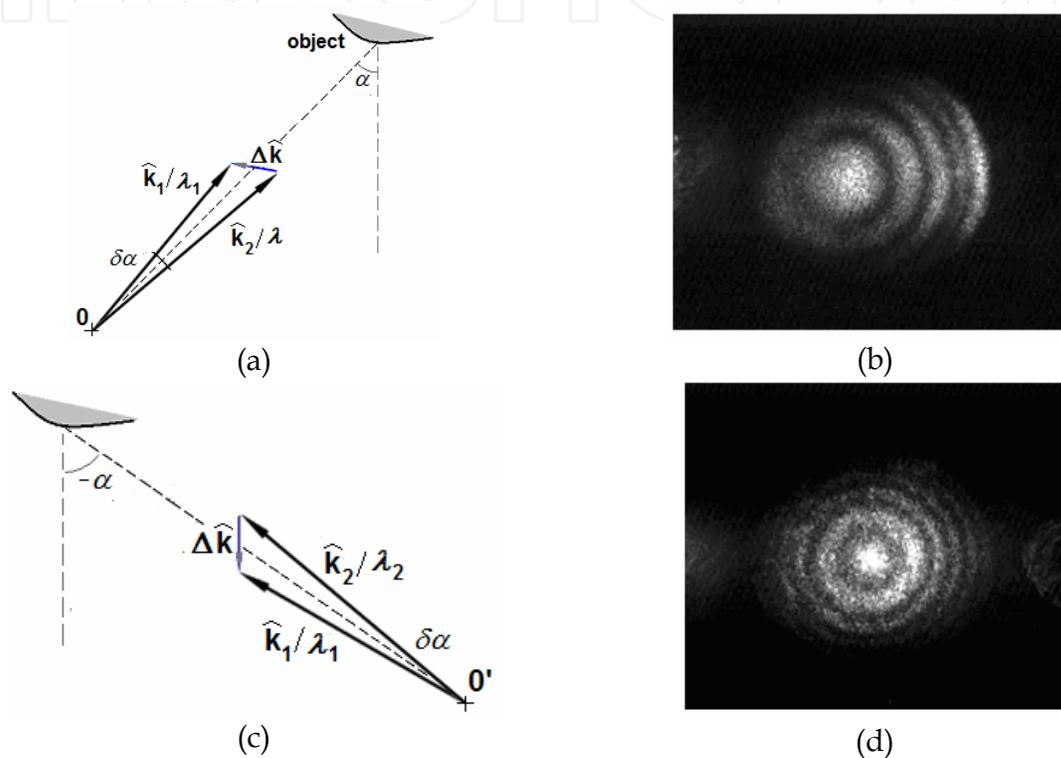
Fig. 10. (a) - Illumination scheme for  $\alpha > 0$  showing the vector  $\Delta\hat{k}$ ; (b) - contour interferogram of the surface obtained with positive  $\alpha$ ; (c) - illumination scheme for  $\alpha < 0$ ; (d) - resulting contour interferogram of the surface with circular concentric fringes (Barbosa, 2010).
