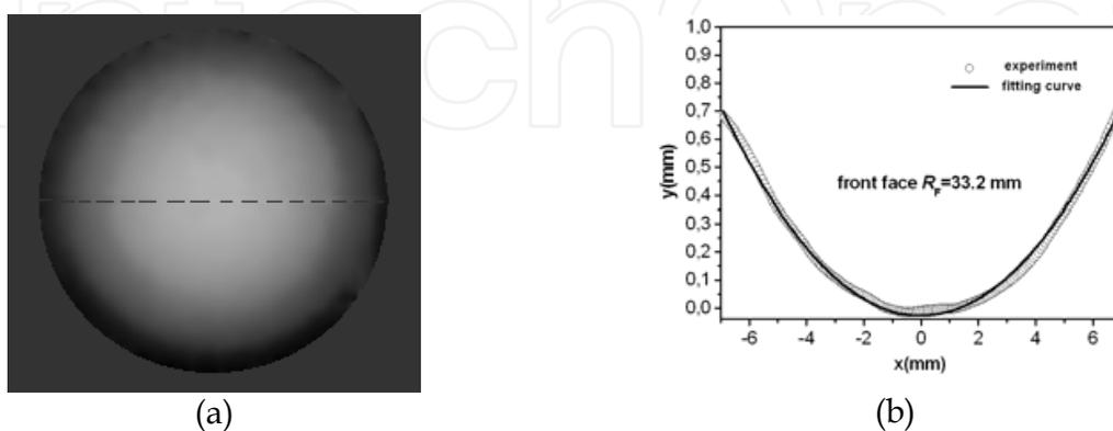
Fig. 16. Reconstruction of the front face of the lens; (a) - unwrapped phase; (b) -  $y$ -coordinate (circles) averaged along radial directions, and fitting curve (black curve) providing  $R_F = 33.2$  mm (Barbosa et al, 2009)
