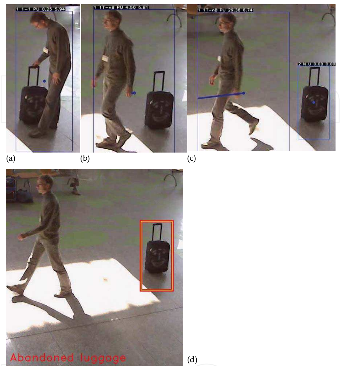
Fig. 14. An example of abandoned luggage detection: (a) initial state, (b) detected left luggage, (c) detected person away form luggage, (d) detected luggage still unattended, high-level event ‘abandoned luggage’ detected, visual alert
