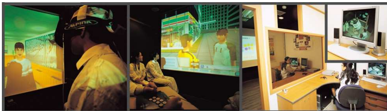
Fig. 1. Virtual reality presentation chamber. The chamber consists of the meeting room and the monitoring room. The meeting room is equipped with a head mounted display, a tracker, a beam projector, a screen, a camcorder, a speaker, and so on. In the monitoring room, a computer system controls all facilities in the meeting room and a situation in the meeting room can be observed through a one-way mirror.
