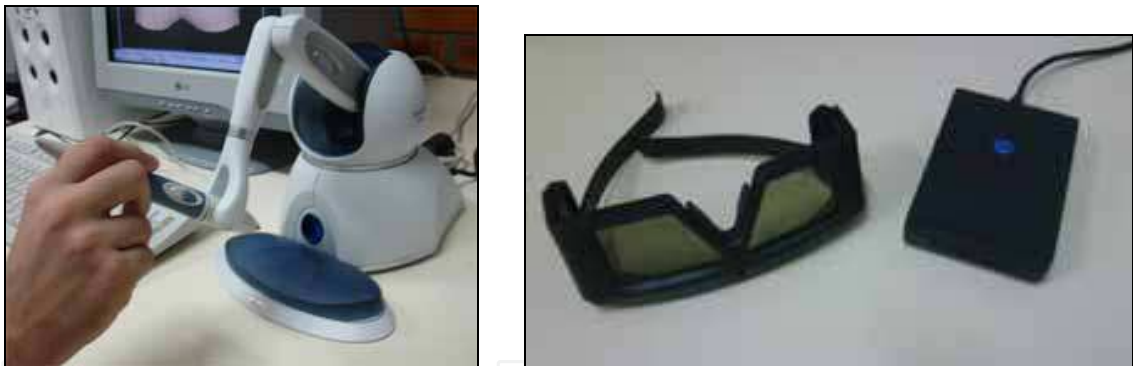
Fig. 5. 6DOF haptic device (left) and shutter glasses for stereoscopic visualization (right). Five models compose the application: three for the human body structures and two for the interaction object. The interaction objects, finger and needle, were modelled with the Blender package and saved in VRML 2.0 format. The models of human body structure were obtained from a previous work (Machado, 2003) and represent the skin of the pelvic region, the iliac bone and the bone marrow (Figure 6). The tissues properties are important information for the simulator. They are used to give to models the same properties of the real tissues. In this case, textures can be acquired or designed, and colours must be defined. Touch properties, as hardness, elasticity and roughness must also be acquired. Because several tissues do not have a numerical value to describe their properties, it is common to acquire them from physicians' impressions. A haptic calibrator was used to do that (Figure 7). Then, some virtual spheres were presented to
