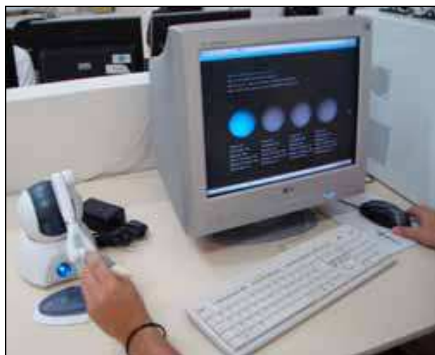
Fig. 7. Tool for calibration of material properties from physicians' impressions.
