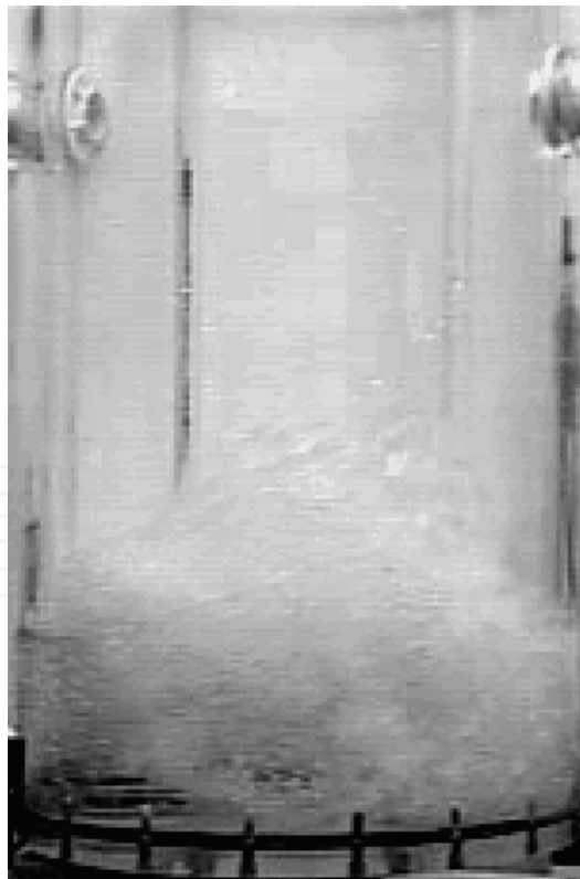
Fig. 12. Images of the vacuum chamber when different nozzles are used. Nozzle Reynolds number \cong 20,000
