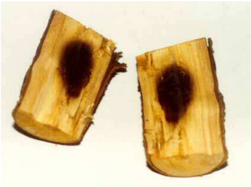
Fig. 11. Charring, due to thermal runaway, in the core of a wood sample that was being dried in a microwave oven (Note: the location of the charring in comparison with the last image in Fig. 7)
