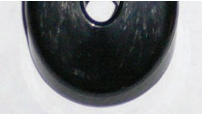
Fig. 3. Warpage and silver streaks at bottle Opener
