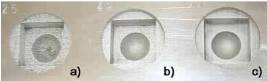
Fig. 12. Workpieces obtained after the operations of roughing (a), semifinishing (b), finishing (c)
