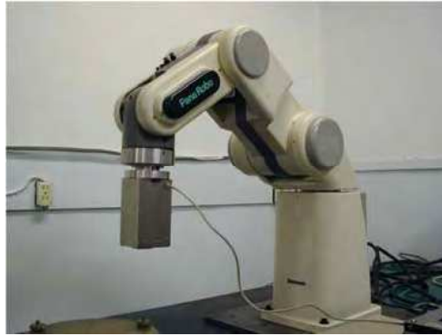
Fig. 4 .Robot equipped with the three-axis tactile sensor.
