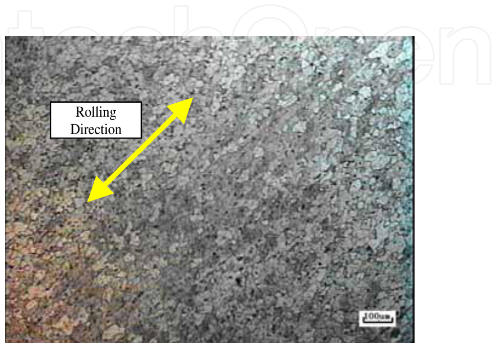
Fig. 6. Microstructure of rolling plate 5052H34
