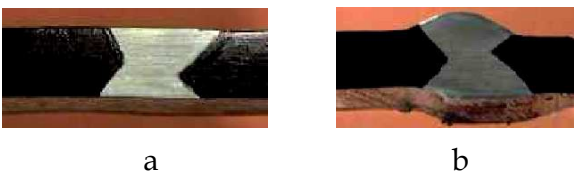
Fig. 16. Toe finish, a) toe emery eliminated, b) bulge emery smoothing.
