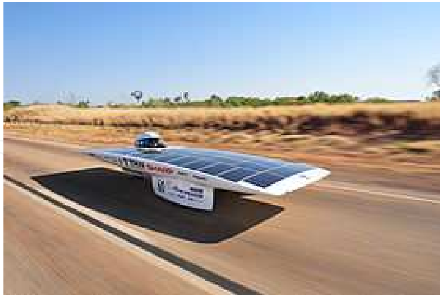
Fig. 5. WSC cars have large areas to place solar panels.
