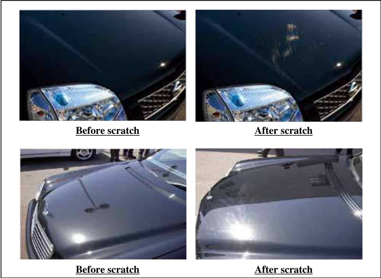
Fig. 4. Visual differences of automotive coating before and after scratching. Mechanical damages of these types may be caused by polishing equipments, carwash bristles, tree branches and sharp objects such as keys (Tahmassebi et al., 2010).
