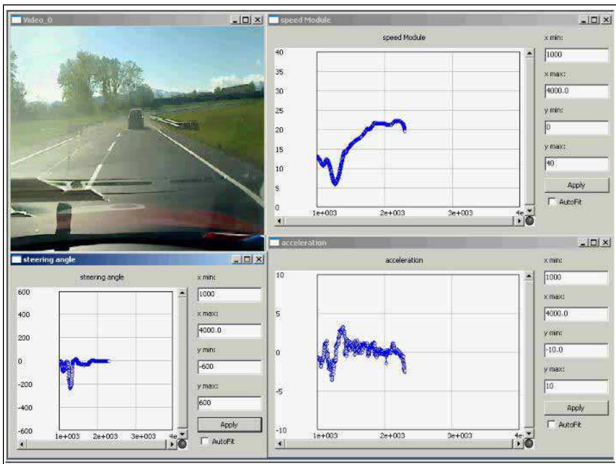
Fig. 9. Video/CAN-bus data visualization
