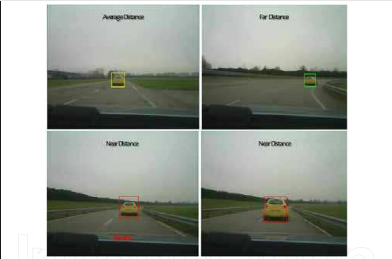
Fig. 10. Dangerous behaviour analysis: an example
