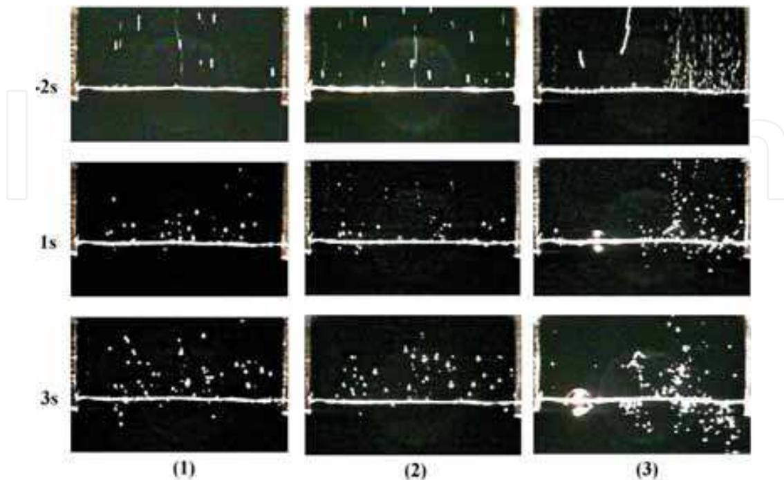
Fig. 2. Bubble behaviors on thin wire in different gravity conditions (Zhao et al., 2004).
