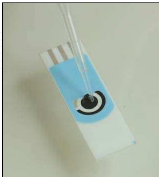
Fig. 8. Screen printed electrode used for biomediator immobilization.
