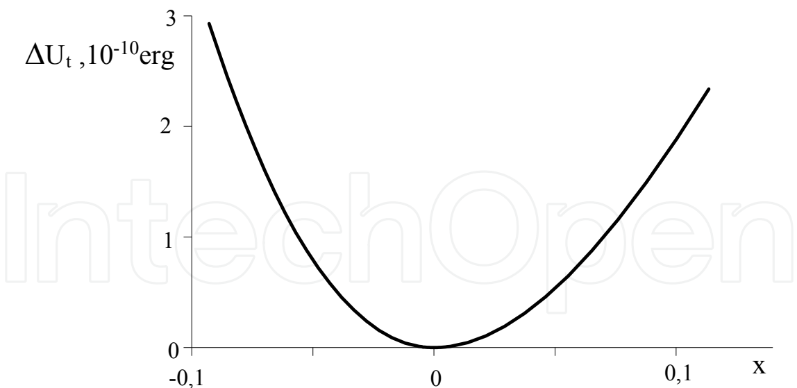
Fig. 4. Variation of the total energy (10 -10 erg) of the cluster vs the relative change of the volume Title of figure, left justified
