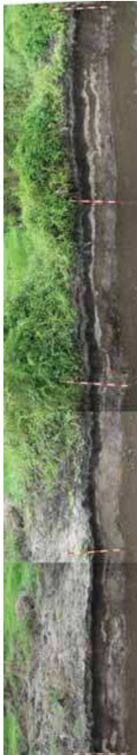
Fig. 11. Trench wall, about 9 meters long, exposing 2004 tsunami deposit (top light colour layer) and up to three paleotsunami layers. The top two paleotsunami sand layers (light colour) are discontinuous, especially the lower one which disappear laterally. Bioturbation and disturbance by animals are thought to be responsible for the discontinuity of this sand layer. The third paleotsunami sand layer is under the water level and only the top edge can be seen in this fig. Stripe on stick is 10 cm.
