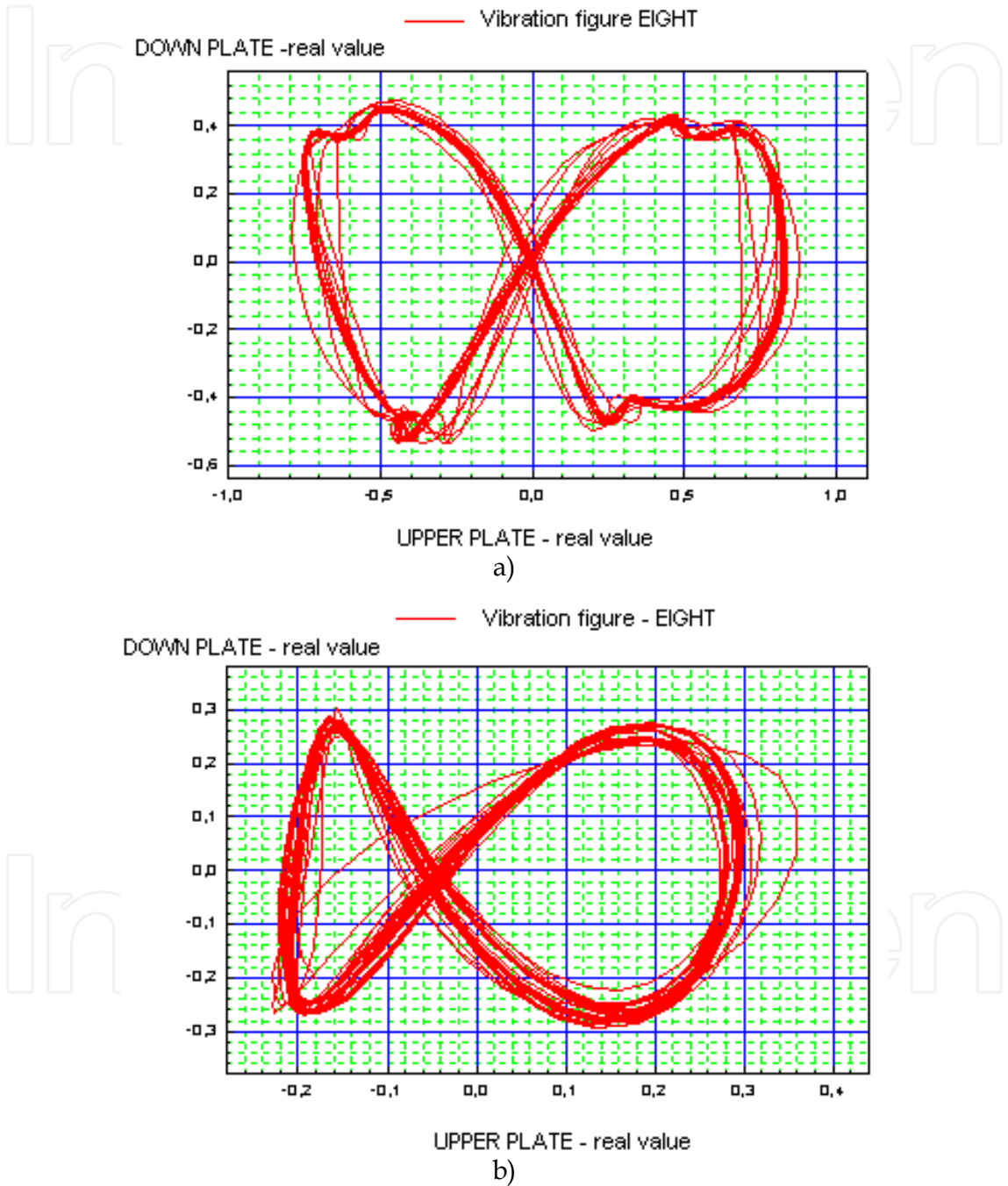
Fig. 6. Vibration figure-EIGHT: a) (1-2 stage; f_D/f_U=4/2 A_D/A_U=1.4/1.4 ); b) (3-4 stage; f_D/f_U=10/5 A_D/A_U=0.5/0.5 ).
