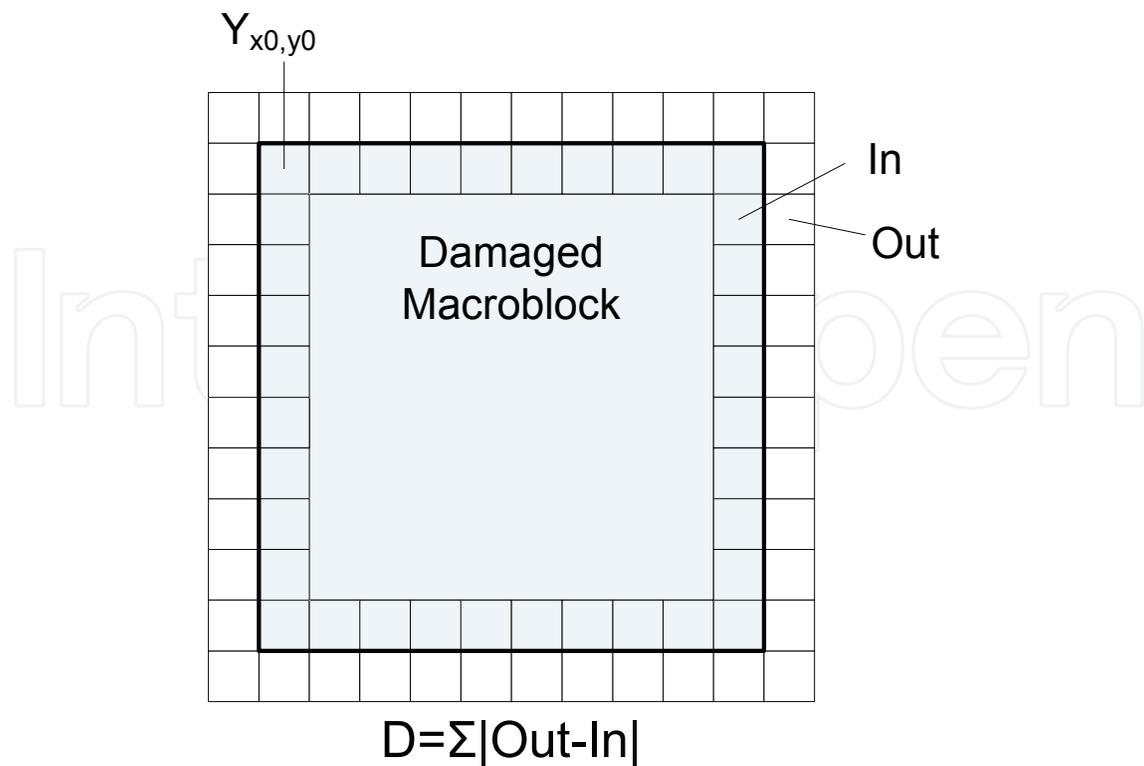
Fig. 4. Side Match Distortion
