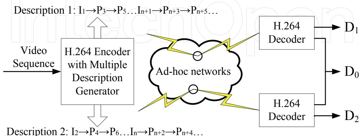
Fig. 1. MSVC system architecture
