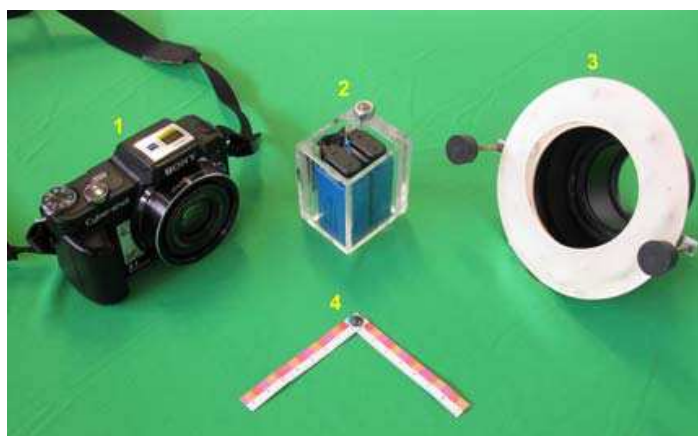
Fig. 3. Current Illuminator prototype. 1: Sony Digital Camera. 2: Illuminator power supply support. 3: Illuminator. 4: Colour ruler (size, colour and focus reference)
