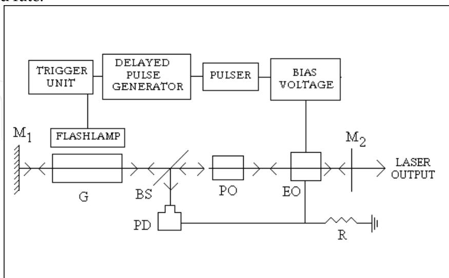
Fig. 6. Block diagram of an electronic pulse stretcher.  $G$ : gain medium of the Q-switched laser;  $PO$ : polarizing optics;  $EO$ : electro-optical device;  $M_1$ ,  $M_2$ : resonator mirrors;  $BS$ : beam-splitter;  $PD$ : photodiode;  $R$ : resistor.
