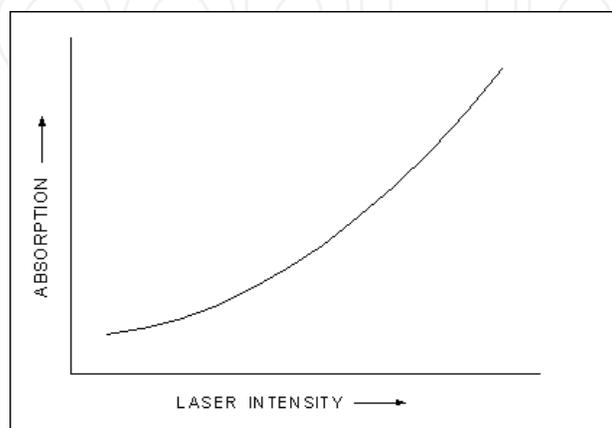
Fig. 5. The absorption characteristics of a nonlinear absorber.
