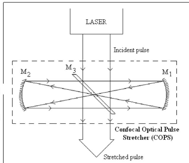
Fig. 2. Schematics of the confocal optical pulse stretcher (COPS).  $M_1$ ,  $M_2$ : 100% reflecting concave mirrors of equal focal lengths;  $M_3$ : partially reflecting plane mirror with a hole at the center (scraper beam-splitter).
