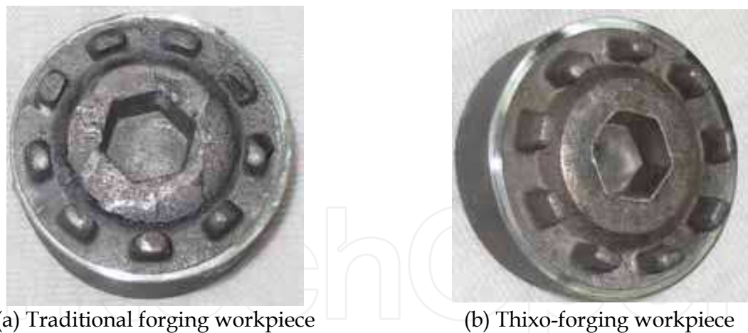
Fig. 11. Traditional forging and thixo-forging workpieces of wrought magnesium alloy
